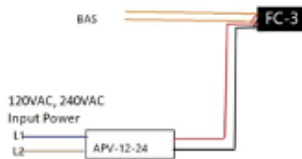
Figure 5: 120V/240V Input Power Wiring Diagram
