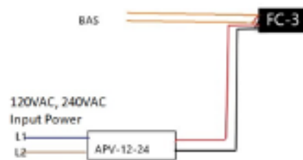
Figure 5: 120V/240V Input Power Wiring Diagram
